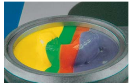
Step 5. For lamination of the next foil - degrease base and model side of the foil and Thermoform! When using multicoloured plates, ensure that the plate is correctly aligned. Allow to cool completely before removing model.
